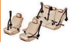
Vehicle three-point pretensioner seat belts
